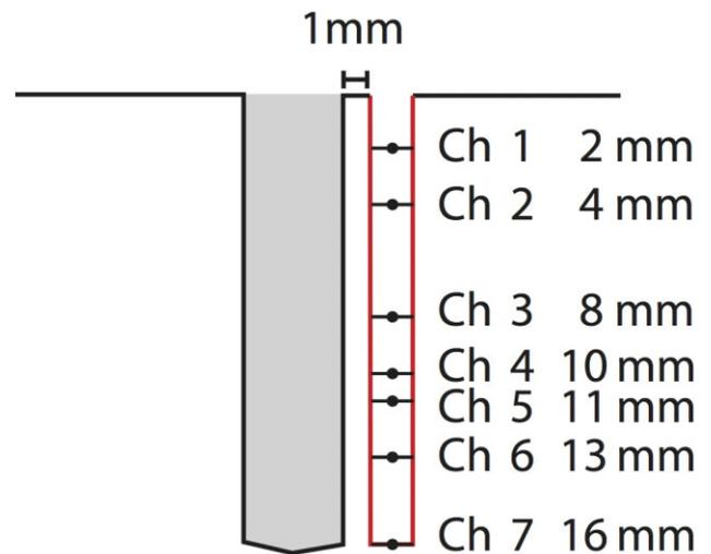
**Figure 1** Schematic representation of osteotomy site and temperature recording by thermoprobe with multiple sensors (Ch 1–4 for 10-mm drilling depth and Ch 1–7 for 16-mm drilling depth).
