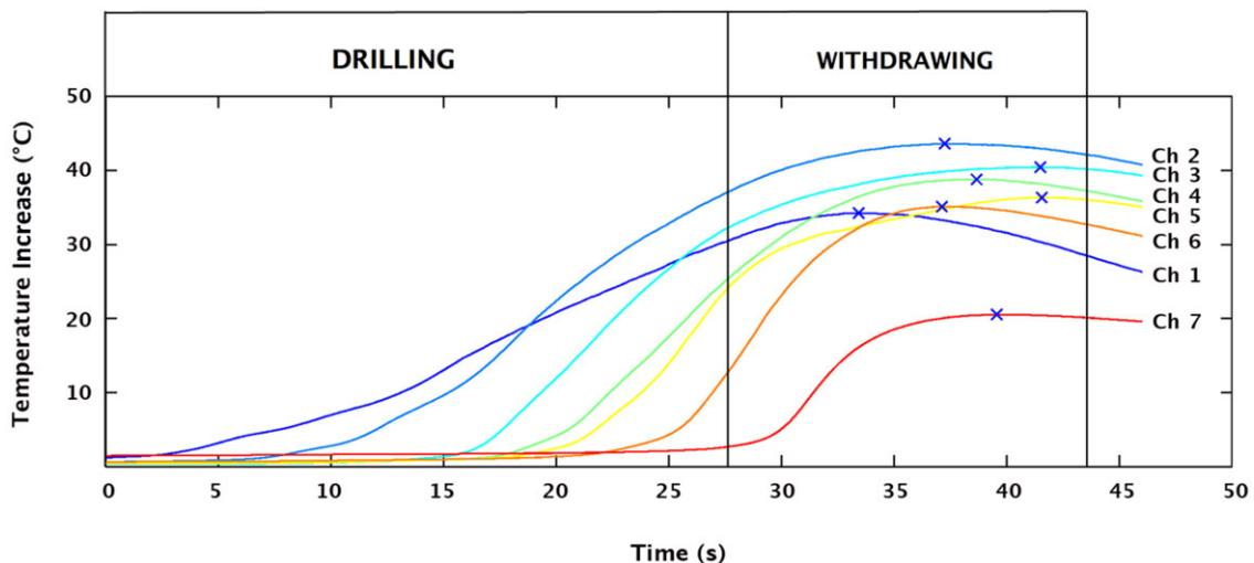
**Figure 3** Illustration of temperature changes during 16-mm osteotomies: recorded in real time by seven temperature sensors at predefined measuring depths; after 27.1 seconds reaching drilling depth of 16 mm ( $\Delta T^{\circ}\text{C}$  at Peak); highest temperature increase (Max  $\Delta T^{\circ}\text{C}$ ) during the withdrawing procedure; x indicates highest temperature increase during the entire drilling procedure.
