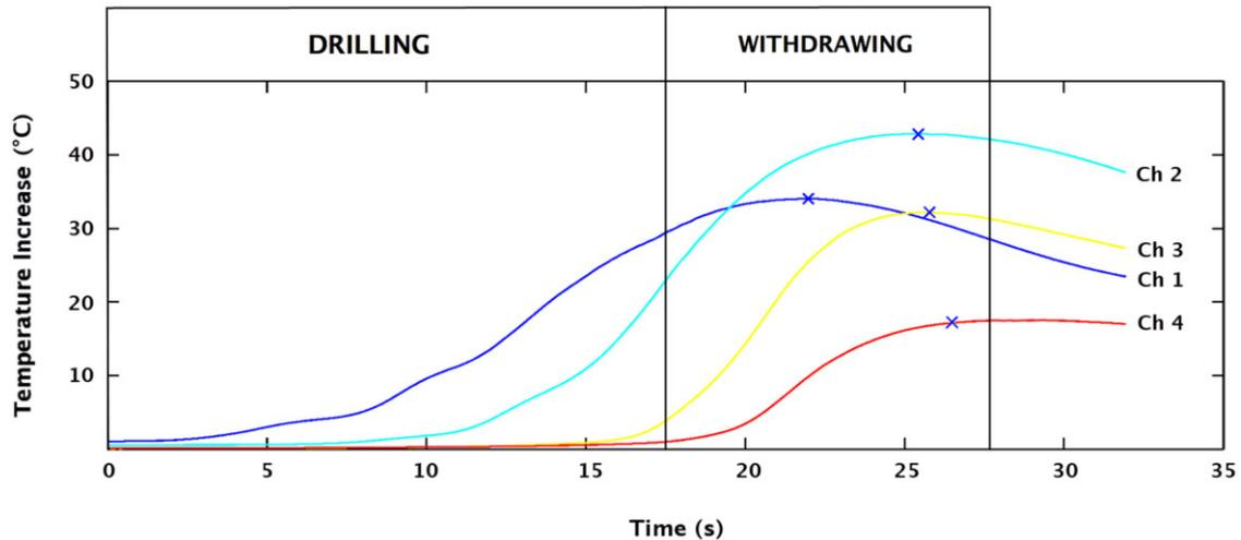
**Figure 2** Illustration of temperature changes during 10-mm osteotomies: recorded in real time by four temperature sensors at predefined measuring depths; after 17.3 seconds reaching drilling depth of 10 mm ( $\Delta T^{\circ}\text{C}$  at Peak); highest temperature increase (Max  $\Delta T^{\circ}\text{C}$ ) during the withdrawing procedure; x indicating highest temperature increase during the entire drilling procedure.
