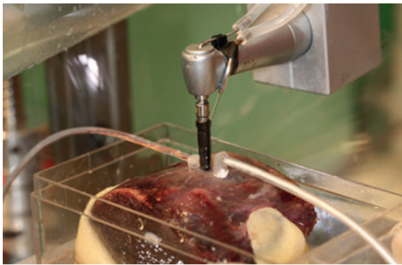
Fig. 7. Automated intermittent and graduated drilling sequence (e.g. 4.3 mm conical implant drill, drilling depth 16 mm and combined saline irrigation) with thermoprobes (SHT 1-Thermoprobe, SHT 2-Thermoprobe).
