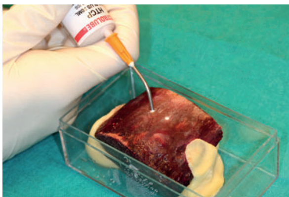
Fig. 6. Injection of a heat-transfer compound (HTCP20S 20 ml, Electrolube®) for an efficient heat transfer during osteotomies.
